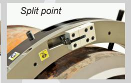
The tool slide performs boring and inside beveling
